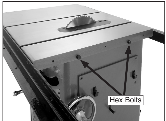
Figure 14. Hex bolts installed.
